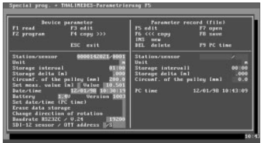
Fig. 13: Configuration window of communication program HYDRAS II
